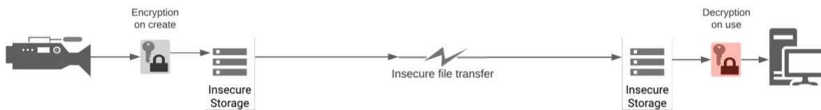
Figure 5-6 End-to-end asset encryption
